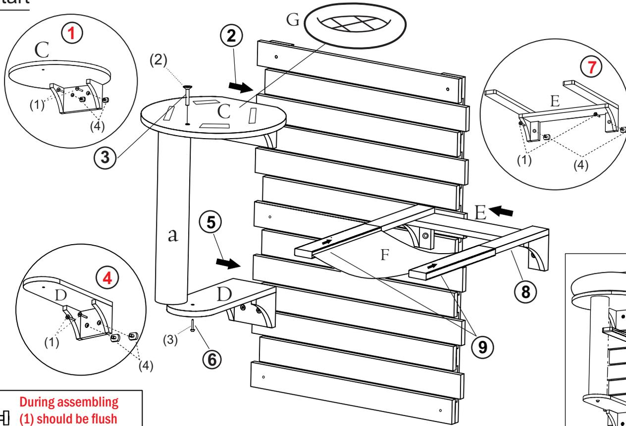
(1) **During assembling (1) should be flush with (4)**
